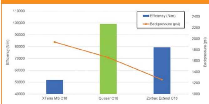
Toluene column efficiency and backpressure for a few C18 columns.
